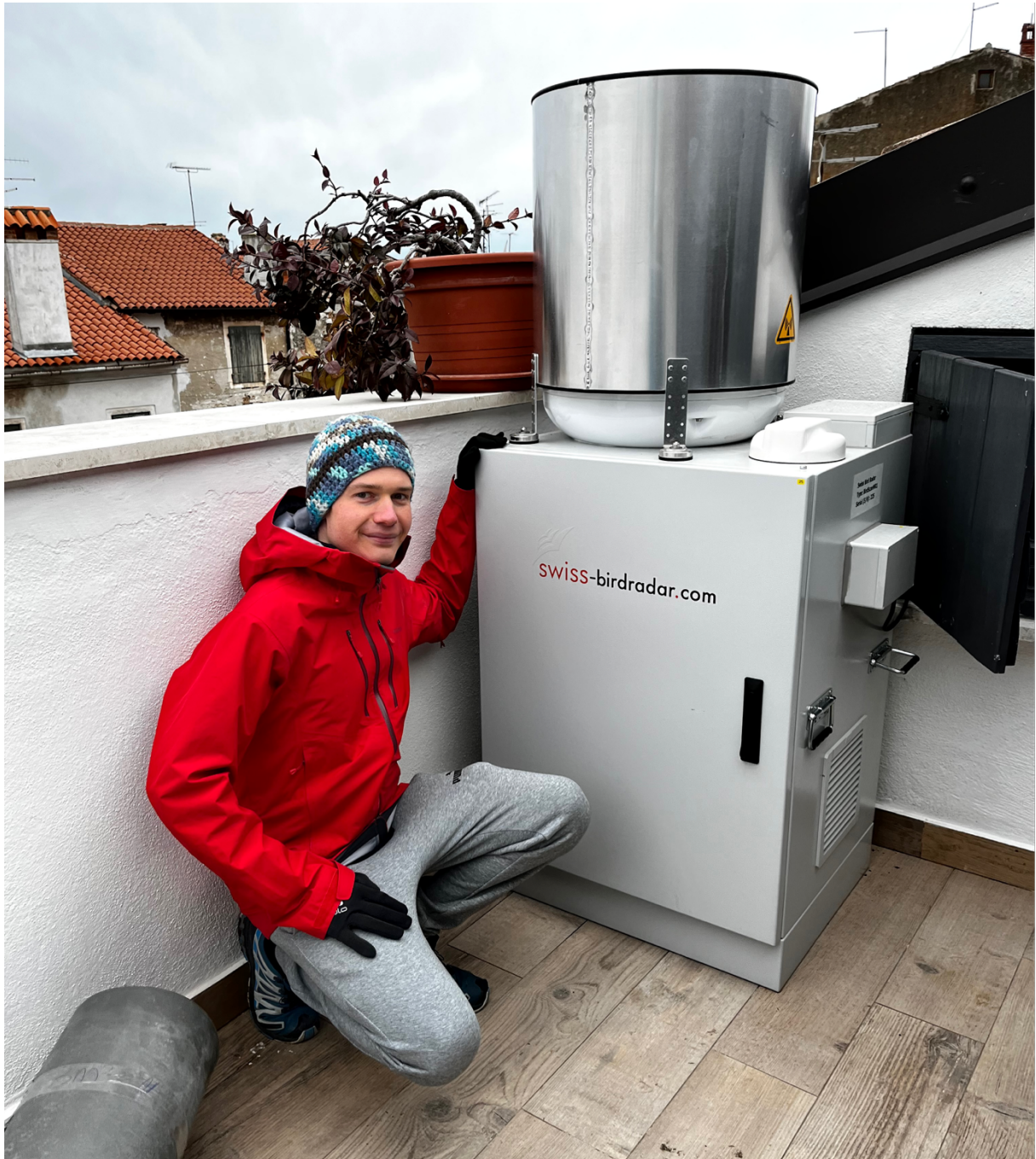
Figure 1.2. BirdScan MR1 during installation at the Rovinj radar site, with the (freezing, but happy) author of this dissertation included for scale. Picture: Barbara Helm.
