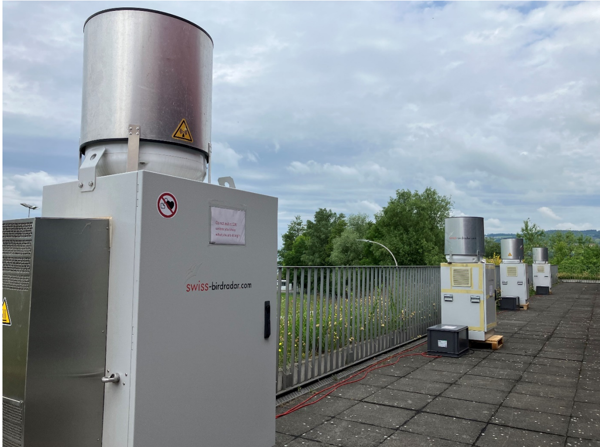
Supp. Fig. A2. Subsequent calibration with parallel measurements of the four BirdScan MR1 radars used in the study, in Sempach, Switzerland, May 2025.
