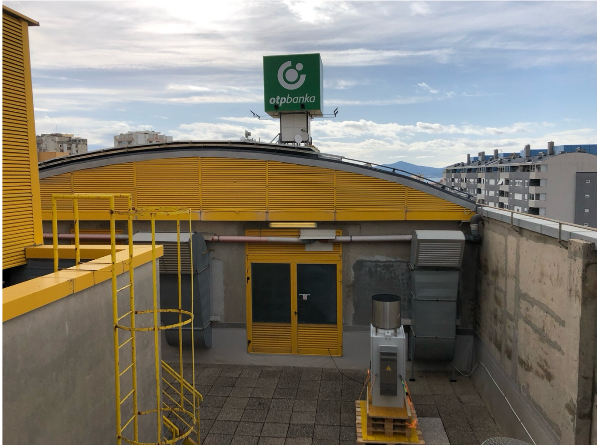
Figure 1.9. BirdScan MR1 in Zadar. The radar was installed on the roof of the OTP bank building, located relatively centrally in Zadar. Due to the metal structures on the roof, the radar had to be placed on wooden pallets to prevent interference with the surrounding building parts. Picture: Simon Hirschhofer.
